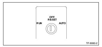
Figure 1-7 Generator Set Master Switch with Keyswitch Option
